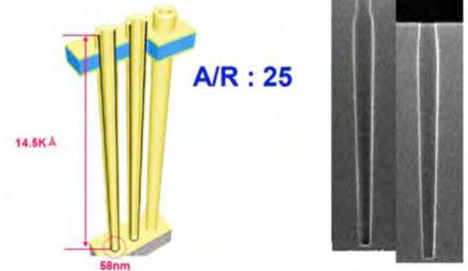
Figure 5. Illustration of the severity of the DRAM capacitor "trench." On the left is a schematic representation of the aspect ratio of a DRAM cell in 3x nm process, showing a "trench" aspect ratio (depth/aperture width) of over 25x. On the right is the actual silicon cross section of two DRAM cells.
